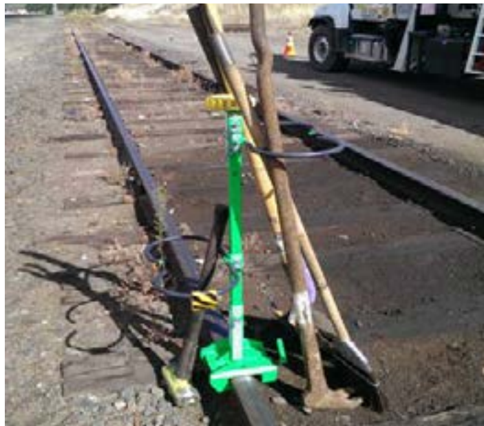
The stand features two adjustable D-Rings to secure both small and large tools.
