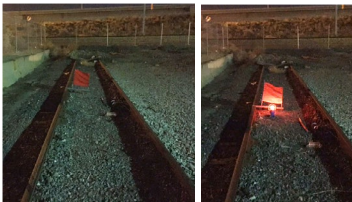
The new derail beacons make it easier to see where a derail is placed. They can be spotted up to a one-quarter mile away.
